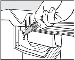
Insert a screw driver into the slot of the emergency opener and pull upwards. The door will now open.
